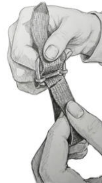
position the folded strap to the bottom side of the buckle
