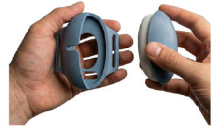
sensor is slid inside the main casing and attached to the charging station
