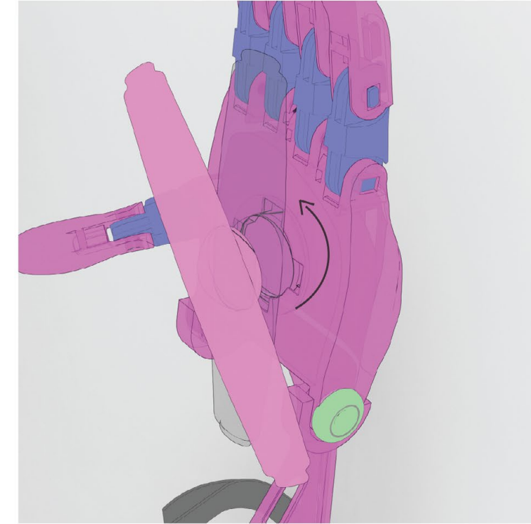
The accessory is rotated and locked in the palm.
